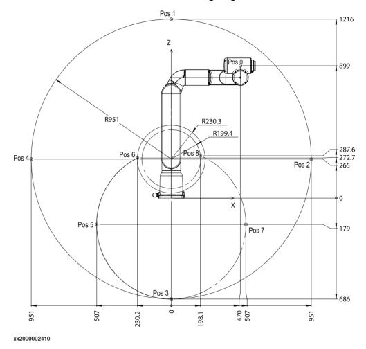
Positions at intersection point of axes 4-5-6 and angle of axes 2 and 3
